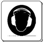
When you use the scarifier BMP-335GHY it is possible to exceed the allowed scale of sound level of 85 db(A). If the scale of sound level reaches 85 db(A) or more, the operators and the persons who work in the surroundings must wear noise protection.
