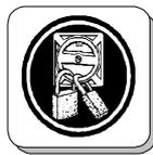
Prior to any repair works on the machine and its drives, secure the machine against unintentional switching-on. Pull out the mains plug or rather the spark plug connector in order to do this.
